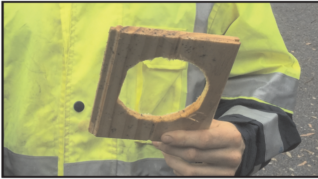
C43rs demonstration cut a 100 mm hole through a 14mm pine timber with 25 litres @ 5000 psi pump
