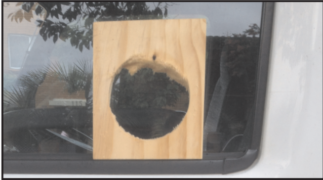
C43rs demonstration cut a 100 mm hole through a 14mm pine timber with a Harben 55 litres @ 4000 psi pump
