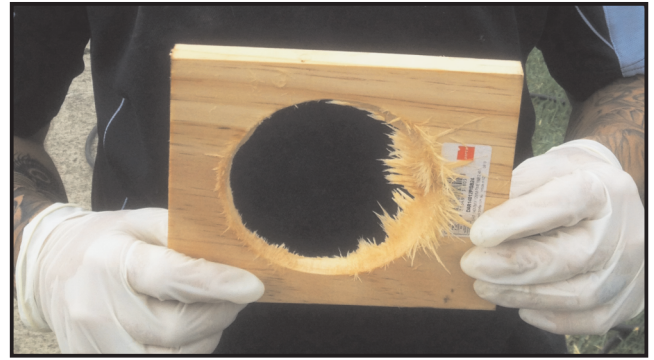
DC38 ring cap and back nozzle demonstration cut a 100 mm hole through a 14 mm timber with a 20 litres @ 4000 psi pump
