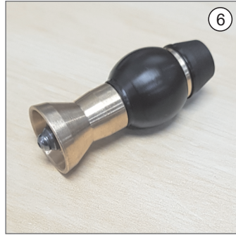
1.Hydro X Nozzle 2.Protective cover 3.Hydro X Nozzle without cover 4.Unscrewed front seat nut 5.Dismantled Hydro X Nozzle 6.Rotor 7.Rubber cone 8.Top insert
